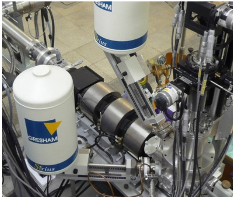
ATOMKI-HAS Oxford-type Scanning Nuclear microprobe.
